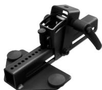
swiveling fastening solution for horizontal and vertical alignment, for flown / ground stacked / mounted applications, incl. accessories (2 x knurled screws M10 x 20 mm, 1 x handle screw M8 x 55 mm), max. load 50 kg
